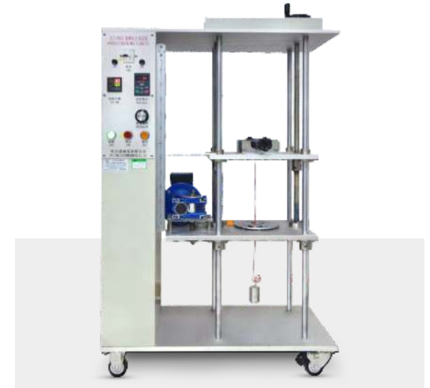
Din Rail Terminal Blocks Rotational Pull Test
