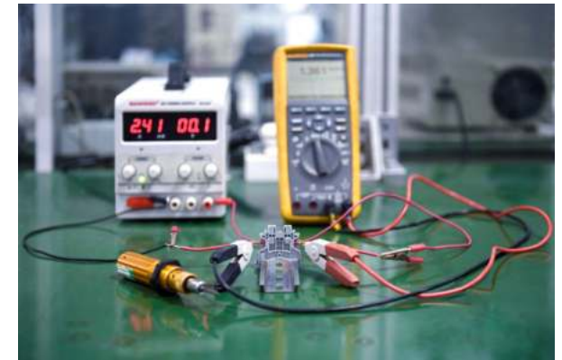
Din Rail Terminal Blocks Voltage-drop Test
