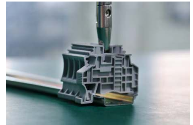
Din Rail Terminal Blocks Touch Protection Test
