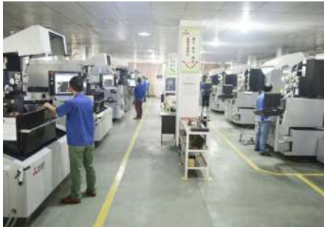
Sodick low speed wire cutting machines(11 sets)
