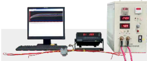
Din Rail Terminal Blocks Temperature-rise Test
