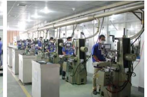
High precision surface grinding machines (30 sets)
