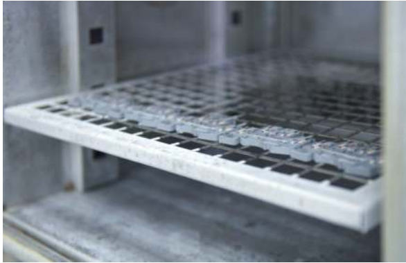
Din Rail Terminal Blocks Temperature Cycling Test
