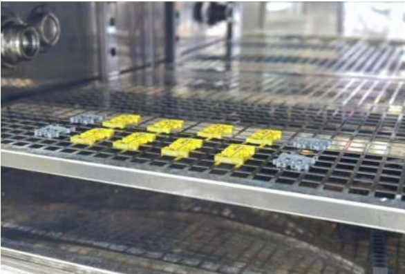
Din Rail Terminal Blocks Temperature Cycling Test
