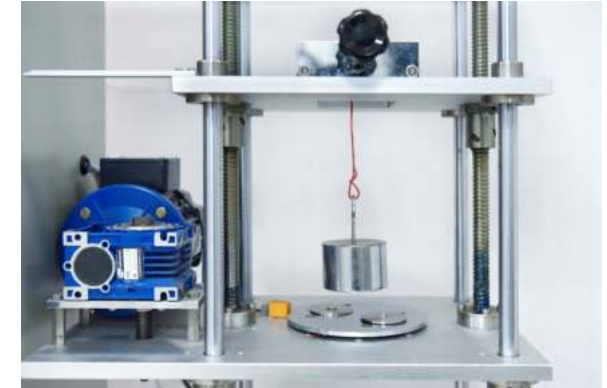
Din Rail Terminal Blocks Static Pull Test
